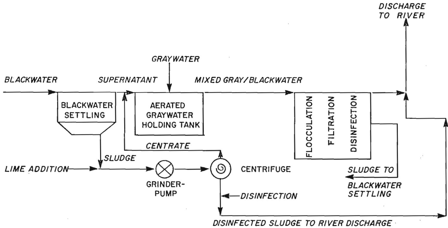
Figure 15. Schematic diagram of modified wastewater treatment system at Emmonak.
