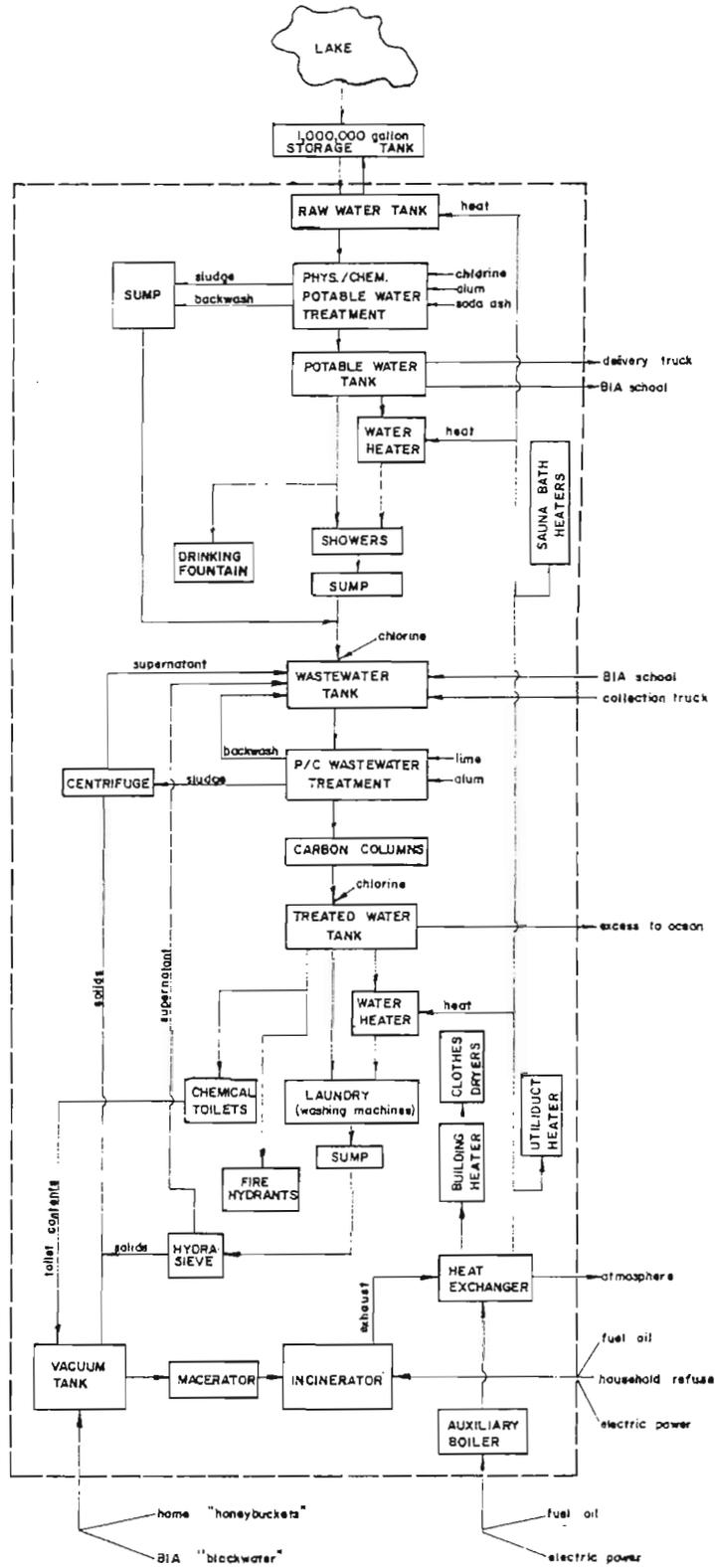
Figure 2. Schematic diagram of project at Wainwright.
