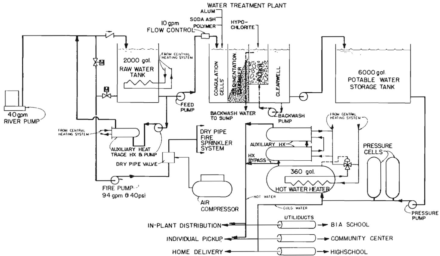
Figure 13. Schematic of water treatment system at Emmonak.
